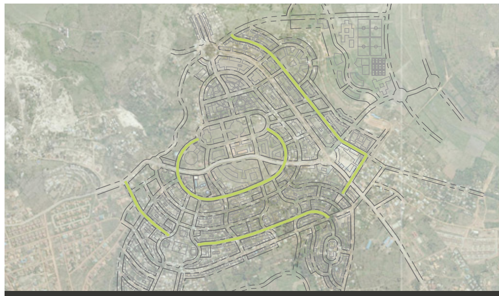
FIGURE 39: GREEN STREETS include landscaped drainage ways that channel and reuse stormwater runoff to create linear parks and urban gardens. The recycling of nature’s bounty is economical because it reduces water usage, reduces erosion, and creates beauty in the city. Above, a map of Kinyinya Sub Area Green Streets.
