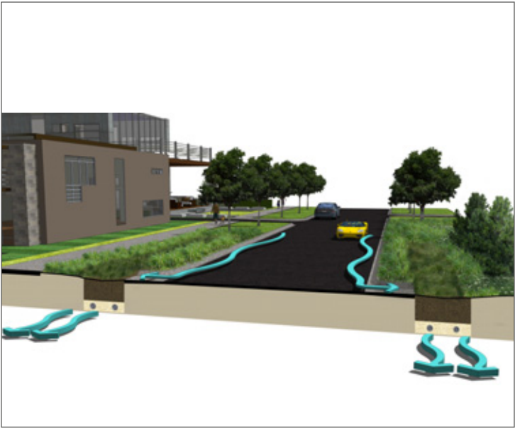
FIGURE 14: URBAN STORM WATER RUNOFF AND DRAIN-AGE systems can utilize water maximally by channelling it through bioswales to irrigate urban landscaping and rain gardens.
