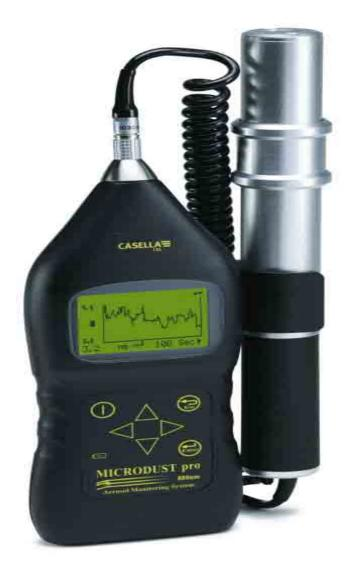
The hand-held, data-logging meter for the real-time detection of airborne dusts, fumes and aerosols is very useful during inspection of demolition sites/mines and construction sites. It has a large LCD display and a unique graphical facility, allowing the user to instantly view the dust level and trends to be compared to admissible intervals. It is ideal for walk-through surveys of ambient and indoor workplace environments.
