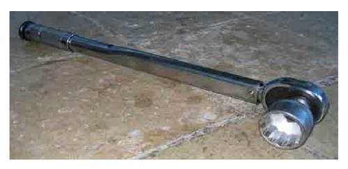
A torque wrench is a tool used to precisely apply a specific torque to a fastener such as a nut or bolt. It was designed to prevent over tightening bolts on water main and steam pipe repairs underground.
