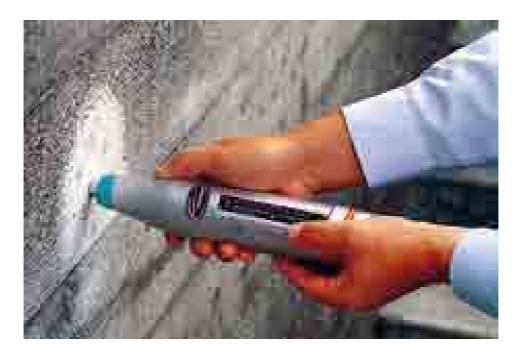
Original Schmidt Concrete Test Hammer
