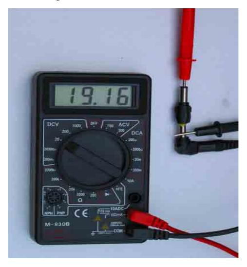
A voltmeter is an instrument used for measuring electrical potential difference between two points in an electric circuit. Analog voltmeters move a pointer across a scale in proportion to the voltage of the circuit; digital voltmeters give a numerical display of voltage by use of an analog to digital converter standards.
