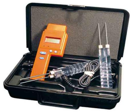
A Digital Moisture Meter Inspection Kit includes everything you need for measuring moisture levels in wood, sheetrock, gypsum, and a variety of other materials with a o to 100 relative scale.
